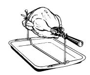
4. Place spit on frame so handle end is in narrow support, and pointed end is in wide U-shaped support.
